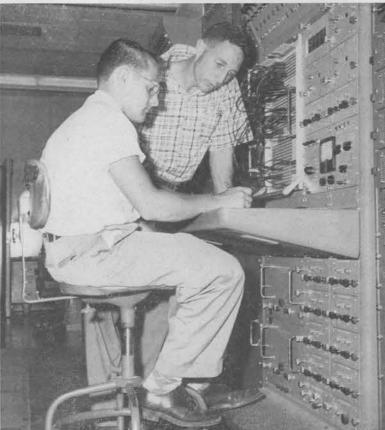
CONTROL PANEL of the analog computer is a maze of knobs, dials, gauges, and patch cords. Here programmers Eugene Aronson (left) and Bob Crabb, both of 5242, go over a problem to be fed into the machine. They can expect the answer in 20 seconds.
